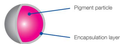
The C7500 uses pigment ink to create fast-drying, long-lasting labels that resist smudging, water and fading.
