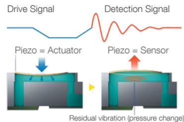
While the printer's Nozzle Verification Technology detects and resolves blocked nozzles, the Dot Substitution feature compensates to help prevent misprints with minimal user intervention.
